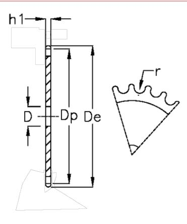
C = 2 D = 30 De = 409.2 Dp = 400.35 For chain size = 3/4 x 7/16 For chain type = 12 B-1 h1 = 11.1 Sumber of teeth = 66
